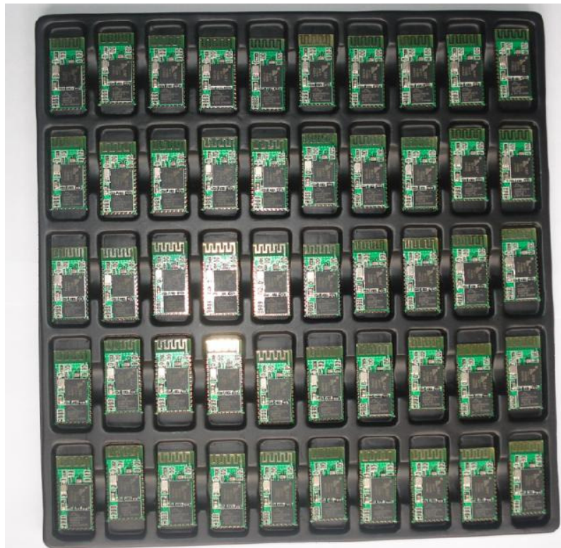
Figure 3 50 pieces chips in an anti-static blister package.
