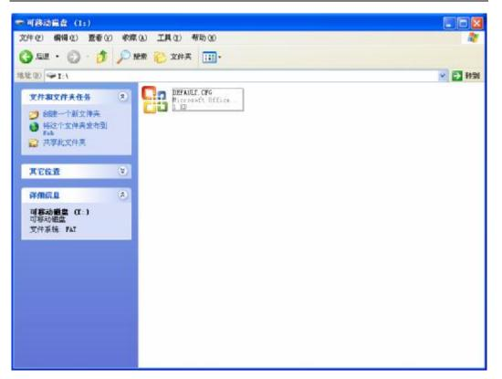
Copy HMSoft.bin file to the disk. After the completion of the copy, HM-15 will automatically restart, then enter the normal working state, the upgrade is complete.
